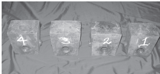
Fig. 5 : Four ADI beater heads having hardness range 370 –440 BHN.
