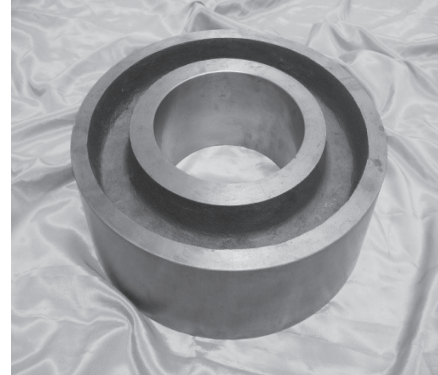
Fig. 16 : Premachined SG Iron Gear Blank Showing Cleaned Machined Surface.
