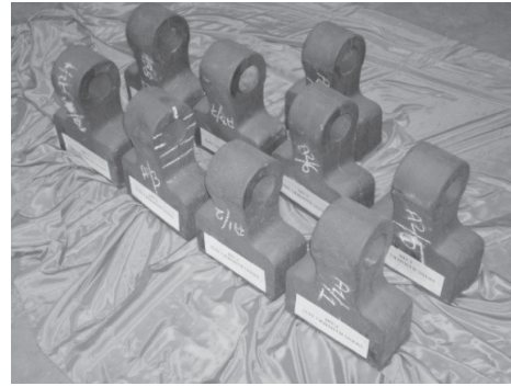
Fig. 14 : Nine Hammers (ADI&CADI) Before Assembly.
