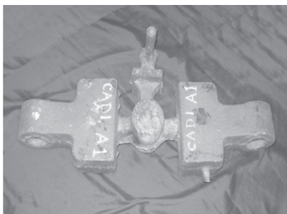
Fig. 12 : As-Cast Hammers with Risers and Runner.
