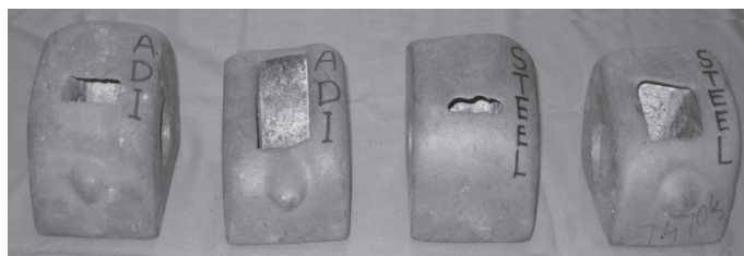
Fig. 6 : ADI beater heads and steel beater heads after 430 hrs of field trials.
