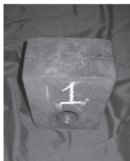
Fig. 4 : ADI Beater head (no shrinkage defect).
