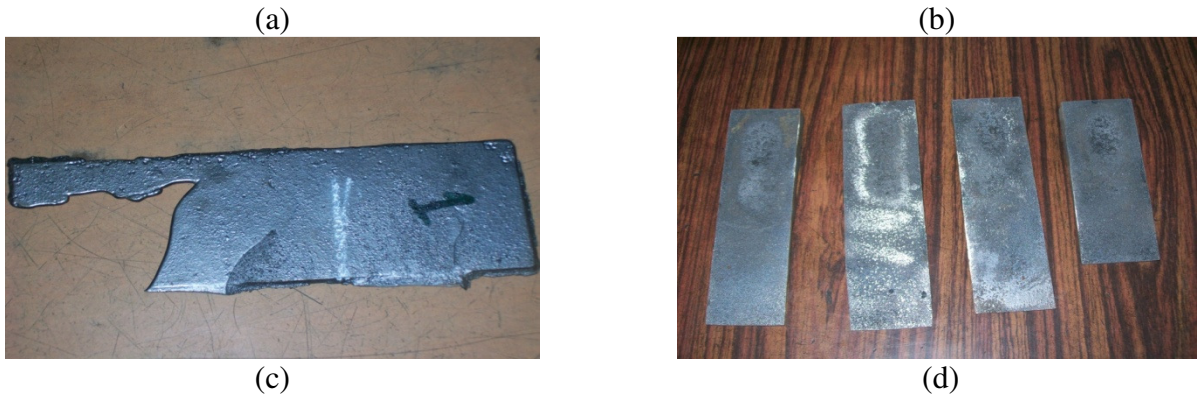
Fig.7 : Casting defects (a) & (b) Cold shut in 3mm plates, (c) Misrun in 2 mm plate and (d) Shrinkage in step bars
