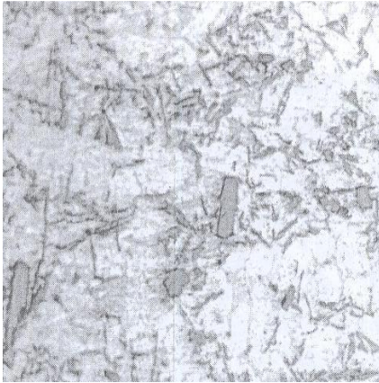
Fig. 9 Optical Micrographs of Alloy B-5 at Different Magnifications (126 ppm P, Pouring Temperature 770°C)
