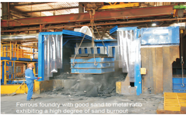
Fig. 2 : Good sand to metal ratio. Ferrous casting exhibiting good burnout of the sand
