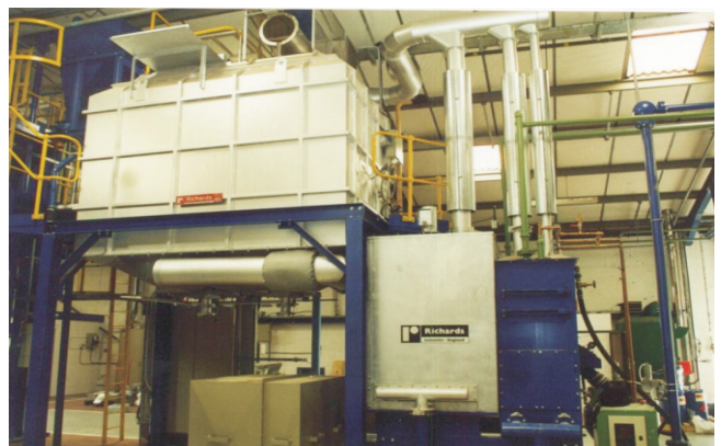
Fig. 5 : Typical Thermal Reclamation Plant
