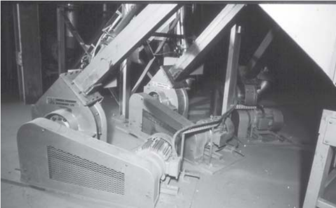
An early form of secondary attrition also known as a 'hammer mill'. This was hard to control and could result in sand grain damage.
