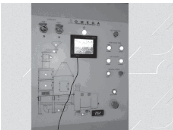
The control panel of the USR monitors the current of both cells and will give warning alarms should the Amperage go outside of preset levels.
