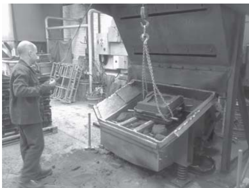
Moulds are knocked out directly onto a 3TPH combination shakeout/reclaimer positioned at floor level.
