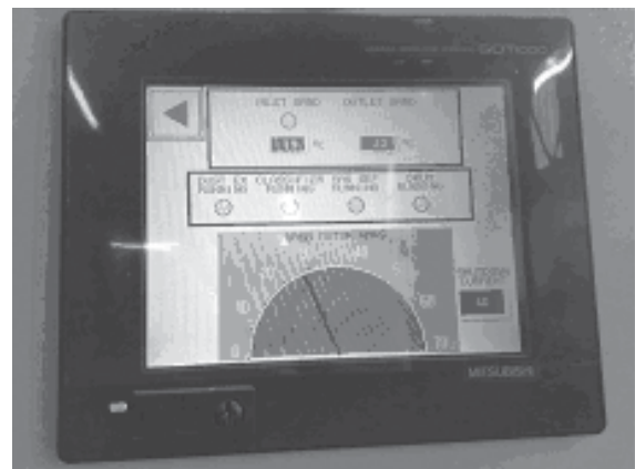
The control panel of the USR monitors the current of both cells and will give warning alarms should the Amperage go outside of preset levels.
