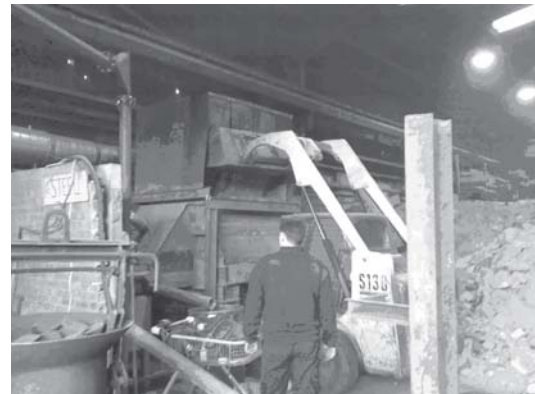
Sand after knockout being fed into the primary attrition mill by payloader.
