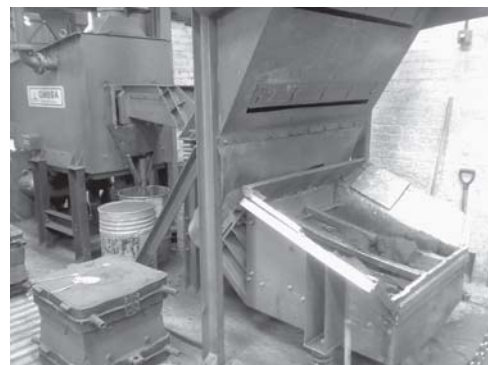
Moulds are knocked out directly onto a 3TPH combination shakeout/reclaimer positioned at floor level.
