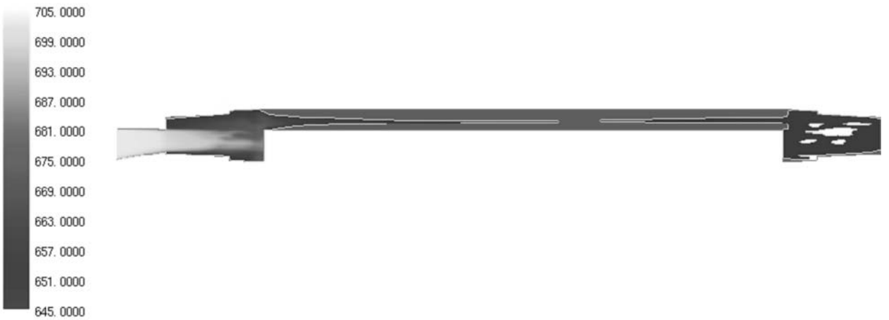
Fig. 6 : Numerical analysis result with misrun (Core length 700mm, slot width 7.6mm, slot length 18.8mm)
