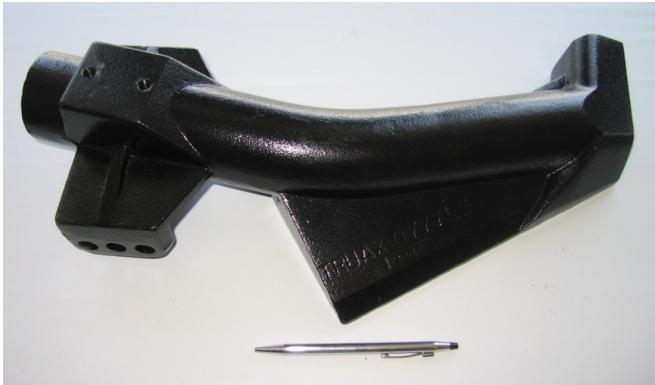
Figure 11: An ADI rangeland seeder boot produced from a green sand ductile iron casting and machined in the as-cast condition.
